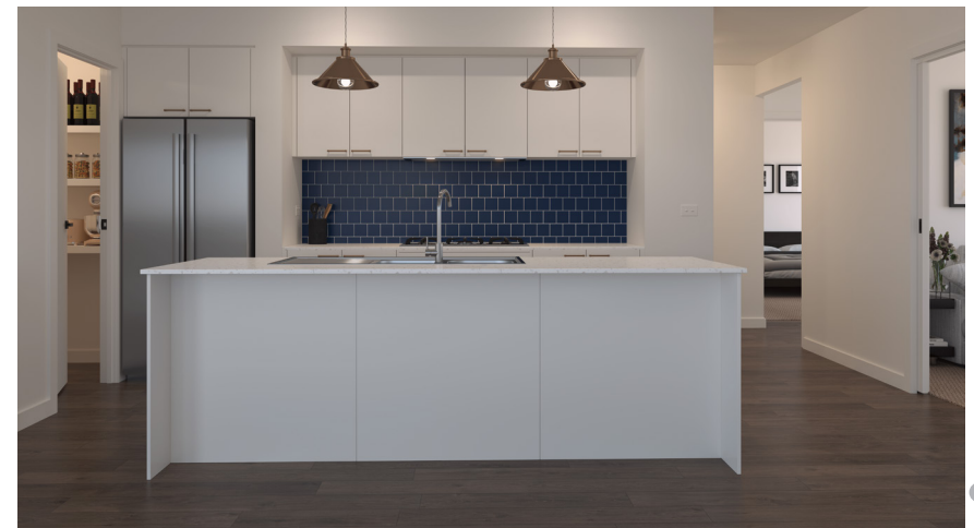
Hamptons Scheme Kitchen: Base & OHC Cabinetry: Formica Warm White Velour, Benchtop: SA White Burst* Handles: SO-3440-160-BN Provincial Brushed Nickel, 128mm to bathrooms. Tiles: SPAWP1043 brick lay
